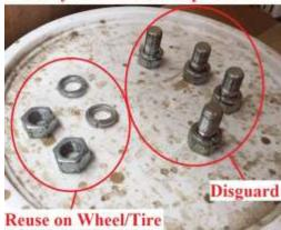
⚠ do not mix these up. You should now have 2 factory nuts/lock washer. Disreguard the 4 factory bolts/lockwasher. We supplied new Lock Washer for the install of the wheel. In Step "H" to install the rim
